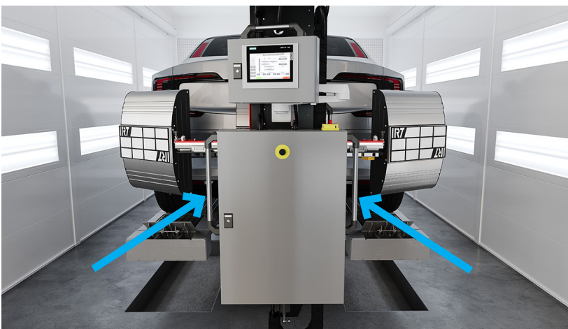
Image above: Use only the indicated handles on the main frame when manually moving ICure.
