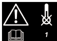
Foutcode 1: Pyrometer defect
