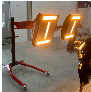
The unique IRT infrared lamps with gold-plated FreeForm reflectors.
