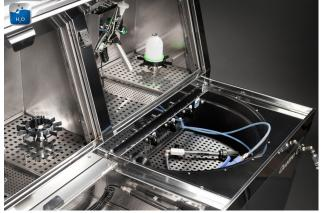
Flow-through brush and rinse gun with recycled waterborne solution. (Tap water optional.) The filtration process separates and dries paint residues to simplify waste handling.
