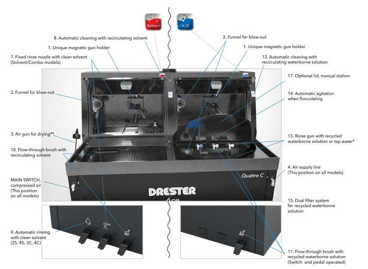
\* Optional watervalve kit for tap water connection including automatic evacuation of filtrate container. Pre-installed: add "T" to item number, e.g. DG2C-T. \*\* (3) Airgun with magnetic attachment can be placed on either side of Ace spraygun cleaner.
