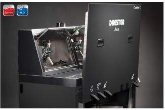
Front cover slides up and rests in service position to allow easy access to solvent/water drums.
