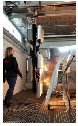
\*It's not an arch, not a half-arch. It is a new, compact I-shaped robotic COMBI dryer. IR and UV curing."
