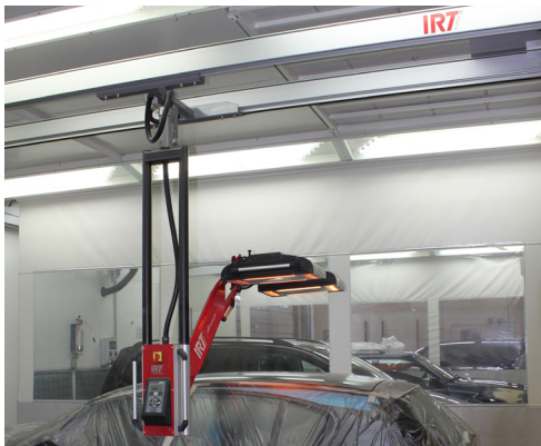
EXAMPLE DRYER IN IRT RAIL
