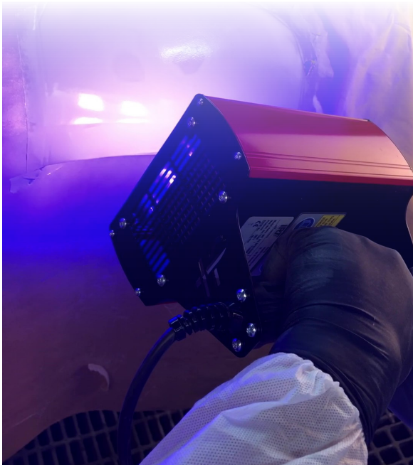
1-2. SPOTCURE ON STAND (OPTIONAL) Combined fixed/handheld curing.
