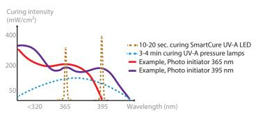
\*Illustrating the correlation between PI wavelength, curing speed and UV-A light intensity.
