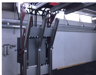
2 distance sensors, 1 measures hood and roof, 1 measures the side.
