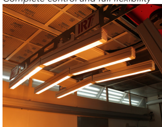
3 IR lamps/zone with a total power of 38 kW.
