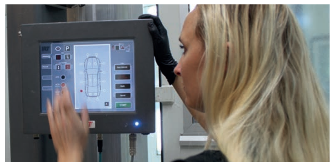
Selection of panels and paint type is done quickly and easily on the touch control panels with user friendly graphics and self-instructive menus.
