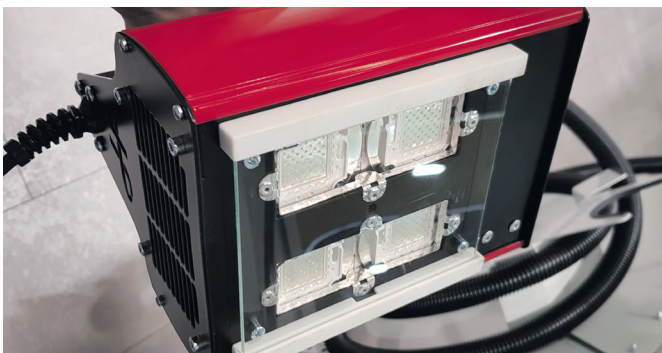
Equipped with four 100W LED modules and protective glass. The glass will prevent the LED getting a dust / overspray-layer on it, resulting in a significant performance loss.
