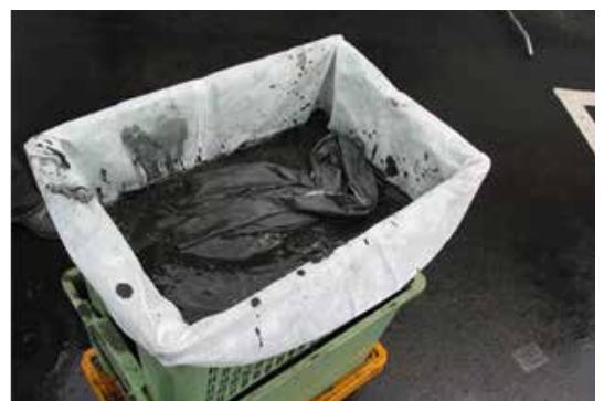
Debris and sludge is collected in the filter basket.
