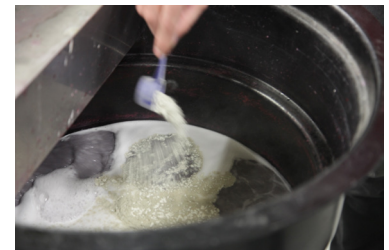
Flocculation powder is added to the water.
