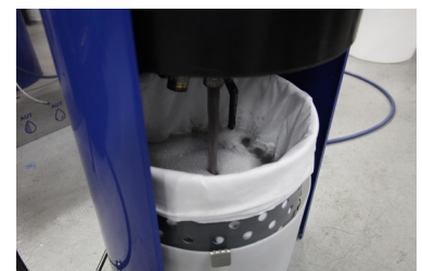
Bottom valve opens to the filter unit.
