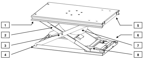
Diagram 8: Lubrication and test points
