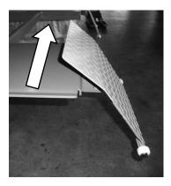
Diagram 6: Elevated lifting platform with mounted loading ramp
