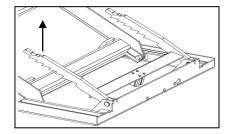
Diagram 4/5: safety catch engaged / safety catch lifted during lowering operation
