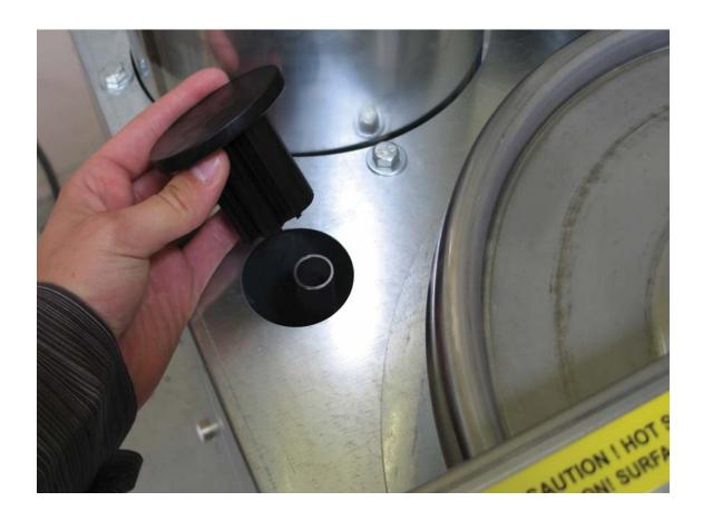
8. Fit the funnel and re-fill unit with the new oil. Pour gently to reduce the risk of accidental overflow. The plastic oil container comes filled with the correct amount of oil for the Drester 10500/10600. Make sure all oil is emptied into the recycler.
