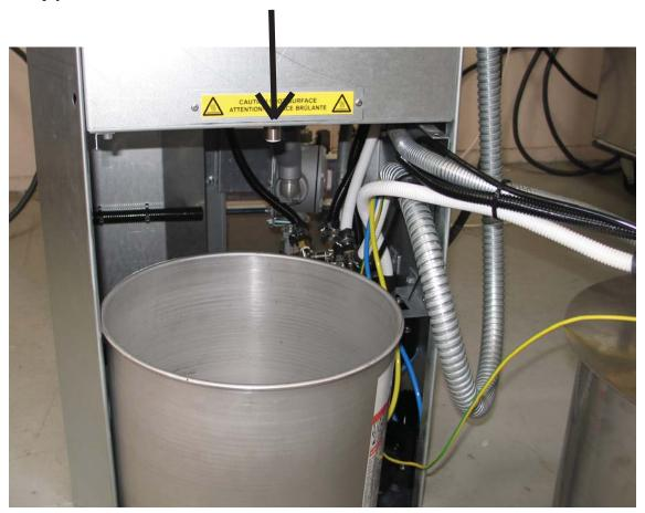
4. Unscrew oil plug and drain oil. Oil plug type may vary (Allen or Hex nut).
