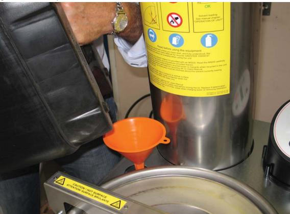
9. Remove funnel and re-fit the oil cap.
