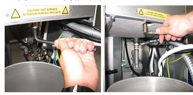
5. Make sure all oil is drained by tilting the unit slightly forward. NOTE: Dispose of old oil according to local rules and regulations.
