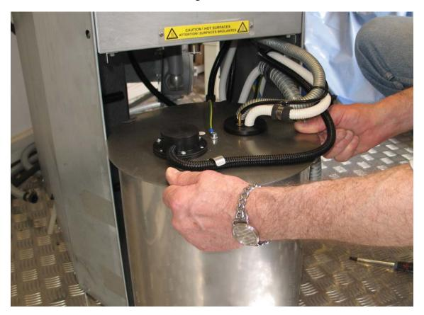
3. Place the empty oil collection drum under the oil outlet.
