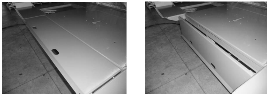
Diagram 7 / 8: Interim drive over ramp in the basic position / interim drive over ramp is folded down.
