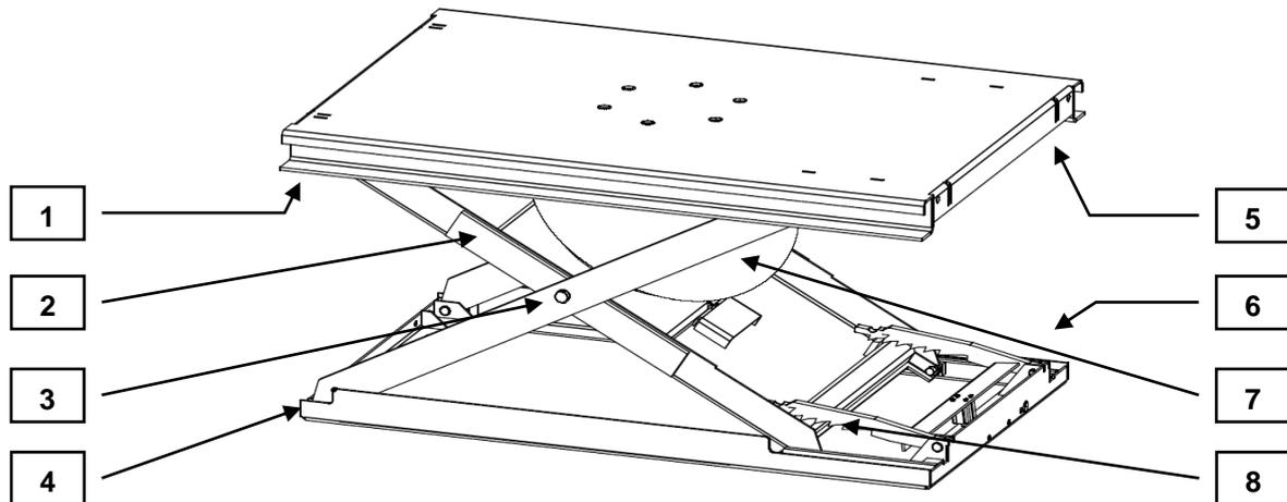
**Diagram 8:** *Lubrication and test points*
