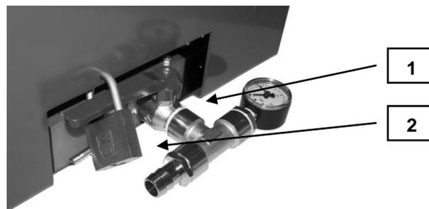
**Diagram 9:** Operating unit is safeguarded from unauthorized use
