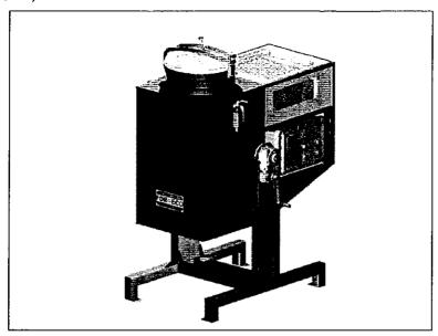
The mixture of solvents with contaminants is brought to boiling temperature inside a boiler equipped with a heating jacket with diathermic oil heated by electric elements. The vapour phase, consisting of solvents, is ducted towards an air cooled or water cooled heat exchanger and condensed; after that the condensed solvent is stored in suitable tanks.
