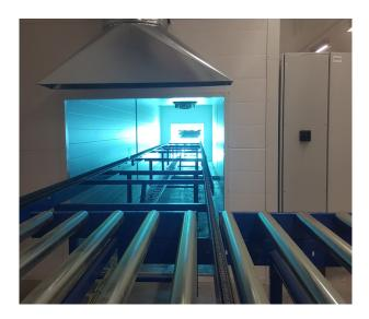
YTAB has 3 lines, the largest 225 m long with an orbit time of approximately 3 hours. Fixtures of plastic parts are installed in a conveyor with 3 basic steps; pre-treatment (static electricity is removed), primer and base coat is applied, clearcoat is applied.
