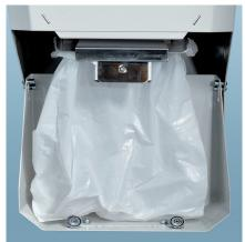
Dust-reduced disposal by opening the sliding plate. The dust goes into the dust bag.
