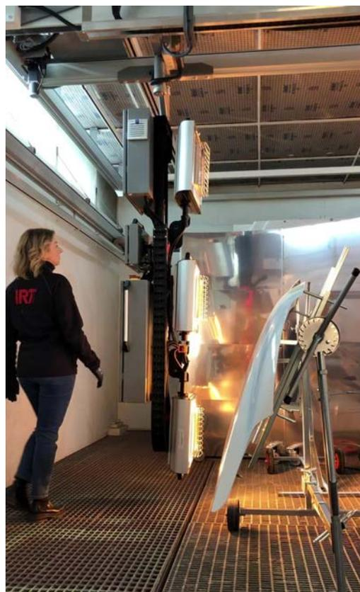
*"It's not an arch, not a half-arch. It is a new, compact I-shaped robotic COMBI dryer. IR and UV curing."*
