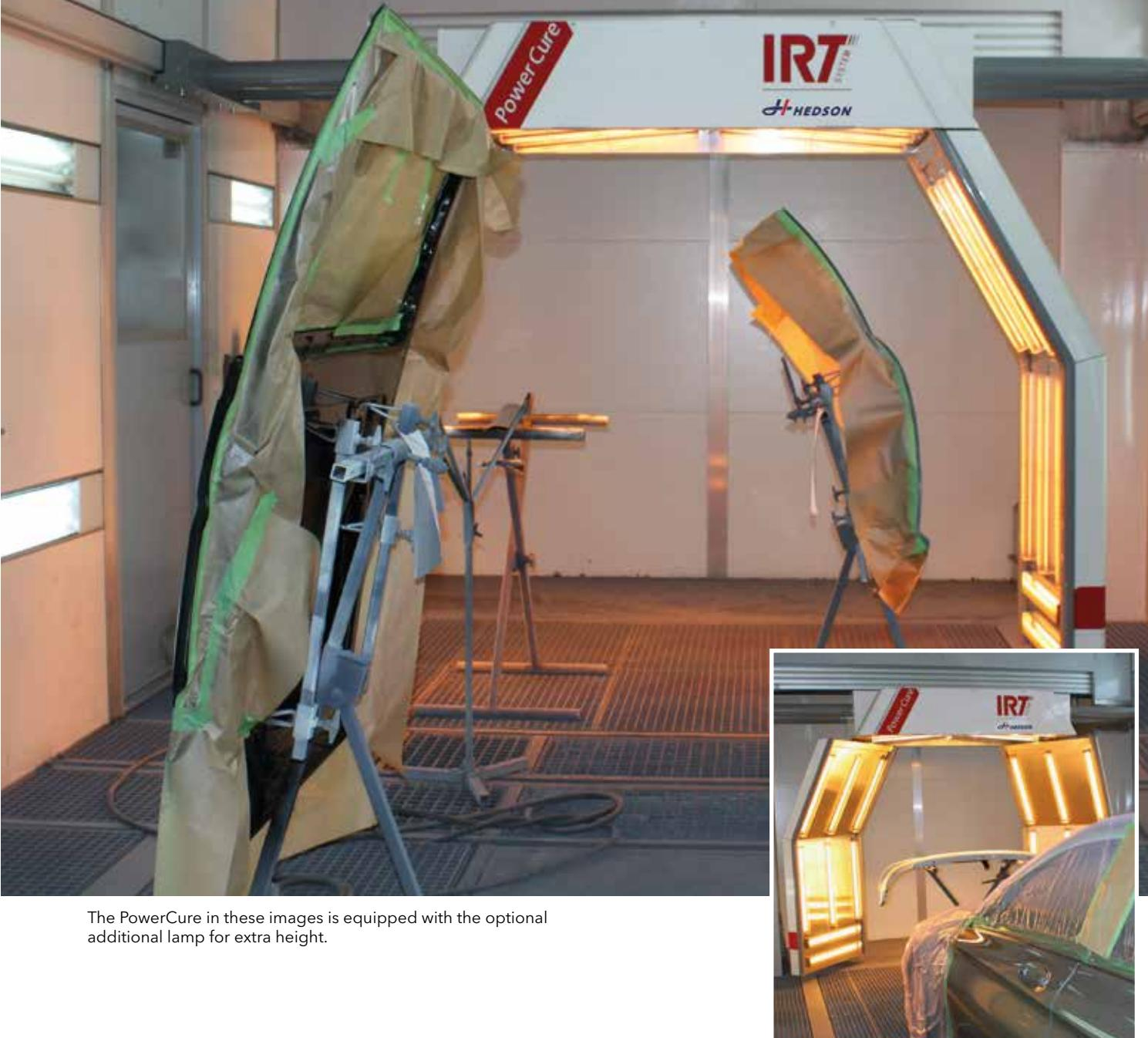
The PowerCure in these images is equipped with the optional additional lamp for extra height.
