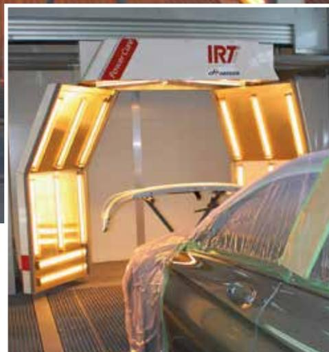
The PowerCure in these images is equipped with the optional additional lamp for extra height.
