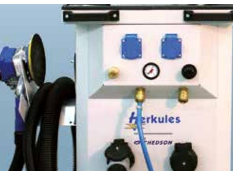
The magnetic equipment holder can be freely positioned to all metal areas.
