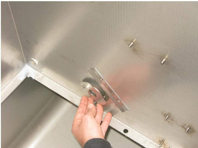
E: Fit the washer. Make sure that it does not “rock” on the bolt heads
