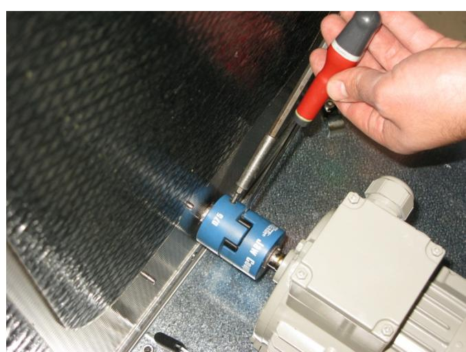
E: Tighten the inner part of the coupling. Make sure there is 1-2mm space between the two coupling parts
