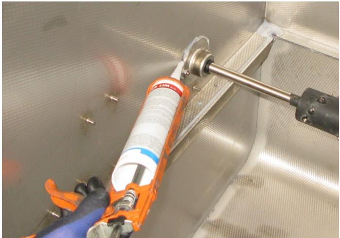
E: Apply silicon around the top edge of the bearing housing
