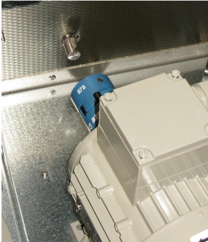
E. Refit the driving motor unit with coupling in place
