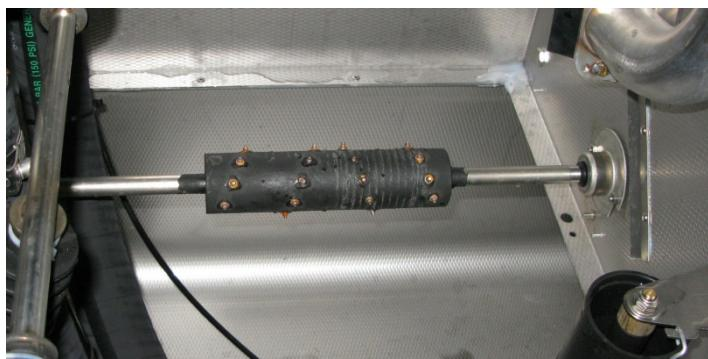
E: Dismantle the 4 nuts (2 on each side) and remove the drive shaft
