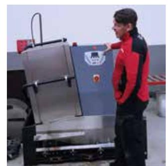
The wheel washer works with a closed water system. This means that the machine can be placed anywhere in the shop. No need for a water connection or a drain next to the machine and the water consumption per washed wheel is only 1 liter per wheel, which we appreciate.
