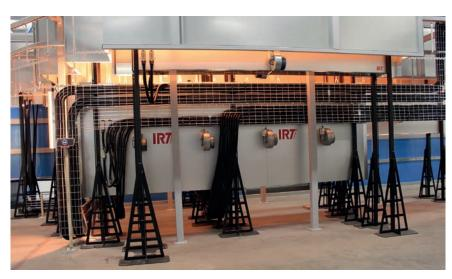
A complete infrared IRT-oven has an extremely short conveyer length. Our IRT-Boosters and IRT-Systems fit in very restricted spaces.
