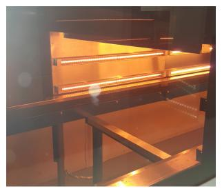
IR-heating is used to create a perfect surface for the chromate conversion top coat, which is cured with UV-radiation.
