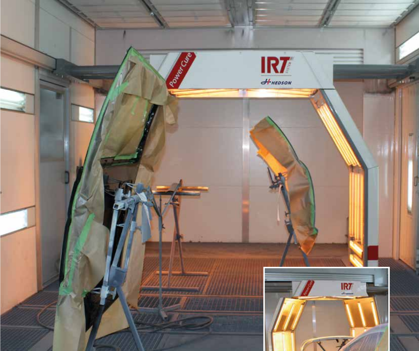
The PowerCure in these images is equipped with the optional additional lamp for extra height.
