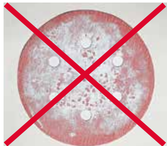
Despite a longer curing time with other products, only the surface is cured and the sanding paper becomes clogged.
